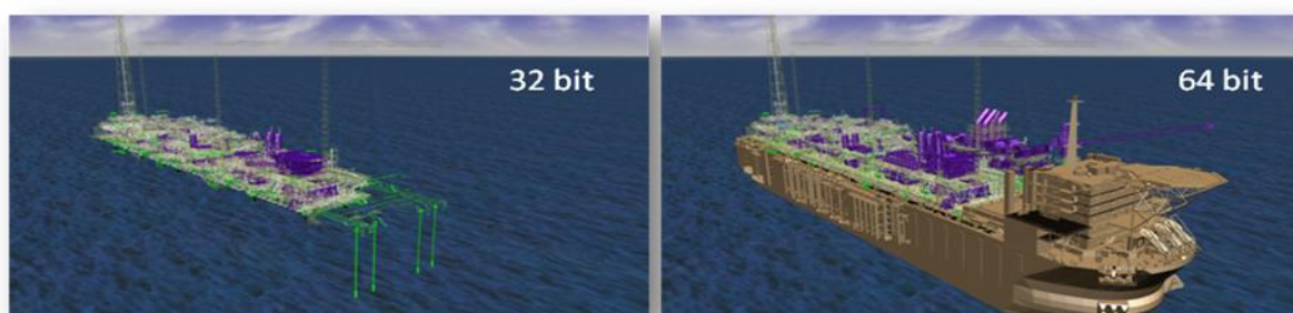
Figure 4: The 64-bit version of AVEVA Review allows more of your model to be loaded
